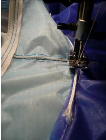
Stitch on a short piece of reinforcement line in the middle at point D. Later on here will be the attachment point for the drogue.
