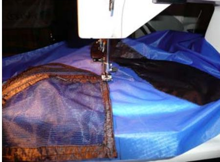
As soon as the back part is completed so far, you can sew the air inlet vent on the appropriate mark.
